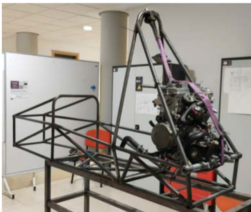
Figura 2. Chasis del FS UCLM Racing Team 2020/21.
