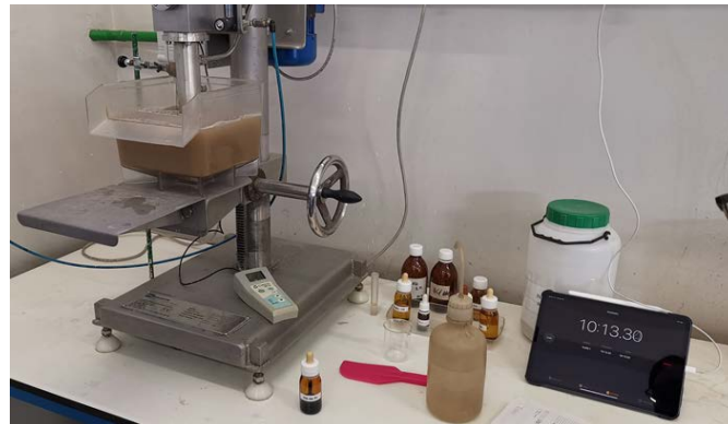
Figure 1. flotation experiment of mixed collectors
