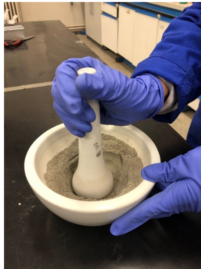
Figure 1. Sample preparation of steel slag
